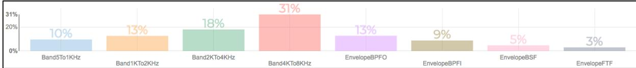
The variables that are displayed in the contribution plot depend on which method in the configured PDX Sandbox project was selected to be the final output for PDX Deploy. For example, if the selected health method is an aggregate of multiple health methods, the contribution variables will be the output of all the health methods. If the selected health method is based on features, then the contribution variables will be the features used for that health method.
